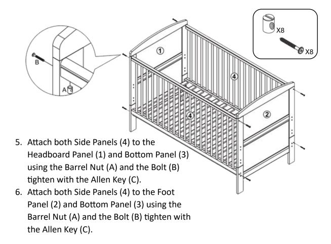
NOTE: The Base Panel can be adjusted as there are 3 height settings, the above shows the lowest.
