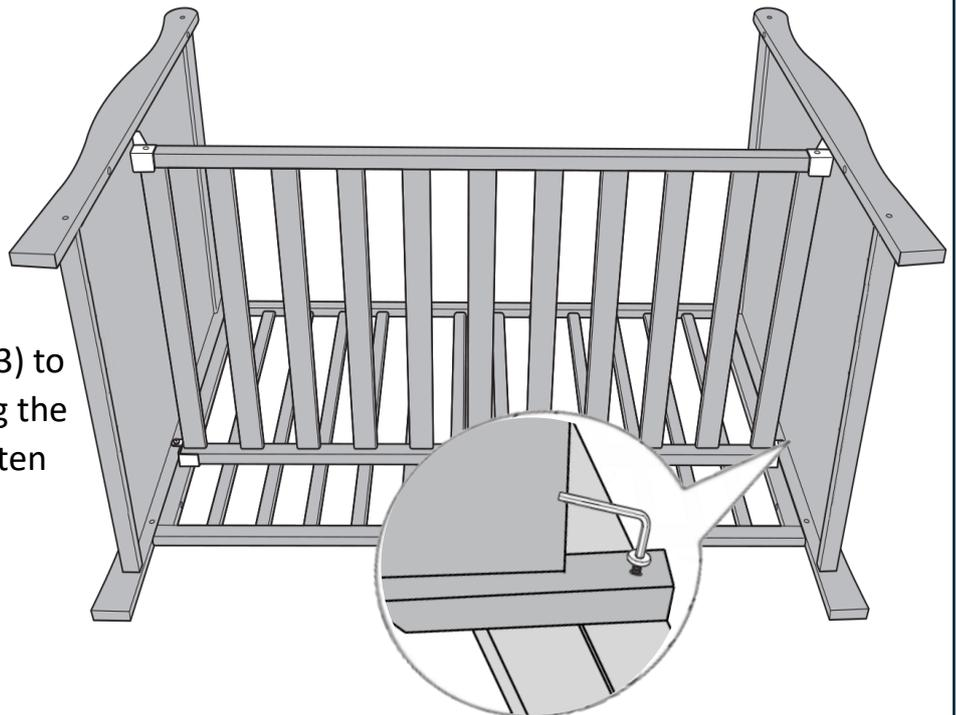
**NOTE: The Base Panel (3) can be adjusted as there are 3 height settings, the above shows the lowest.**
