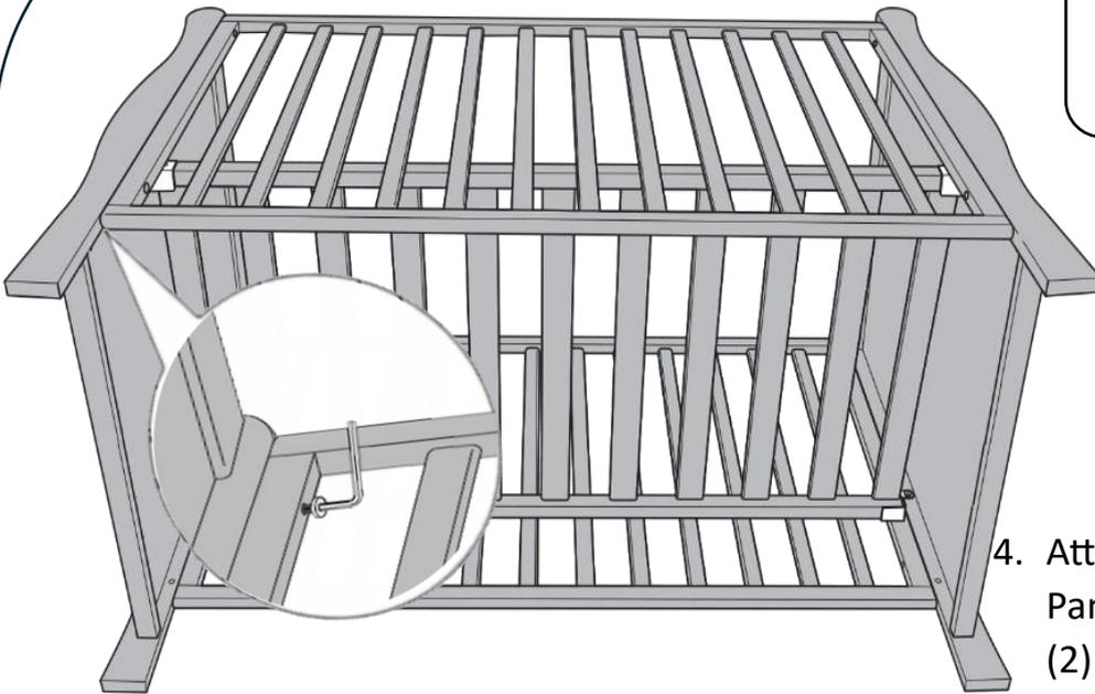
4. Attach the remaining Side Panel (1) to the End Panels (2) using the Long Bolts (A) and tighten with the Allen Key (C).
