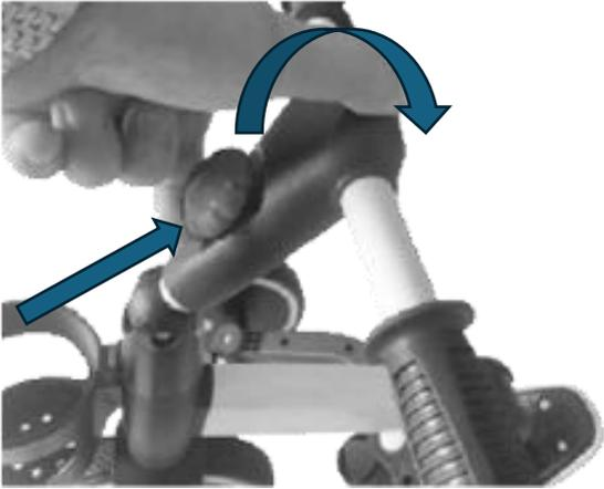
1. Loosen the button on the Handlebar (B), by turning anti-clockwise and lift upwardly. The Handlebar (B) can now be folded as shown below.
