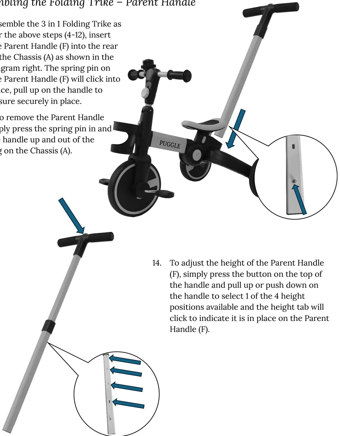
14. To adjust the height of the Parent Handle (F), simply press the button on the top of the handle and pull up or push down on the handle to select 1 of the 4 height positions available and the height tab will click to indicate it is in place on the Parent Handle (F).
