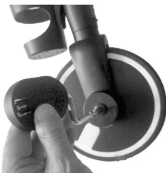
12. Press the button located beneath the housing of the Front Wheel (D) and insert the pedals. You should here a click to confirm in place, however pull on both pedals to ensure in place securely.
