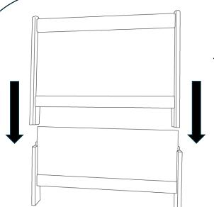
7. Remove the bottom section from the Headboard/Foot Panel (2).
