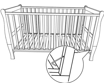
NOTE: The Base Panel can be adjusted as there are 3 height settings, the above shows the lowest.
