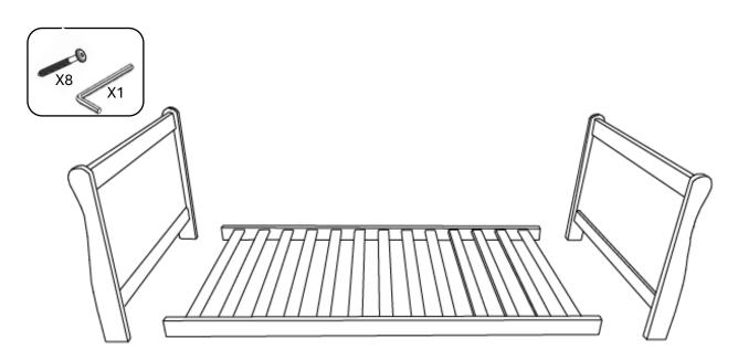
9. Attach the top section of the Headboard/Foot Panels (2) to the Base Panel (5) using the Short Bolt (B) and tighten with the Allen Key (C).
