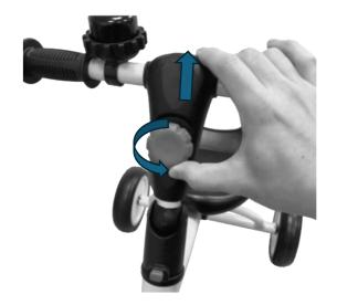
1. Loosen the button on the Handlebar (B), by turning anti-clockwise and lift upwardly. The Handlebar (B) can now be folded as shown below.
