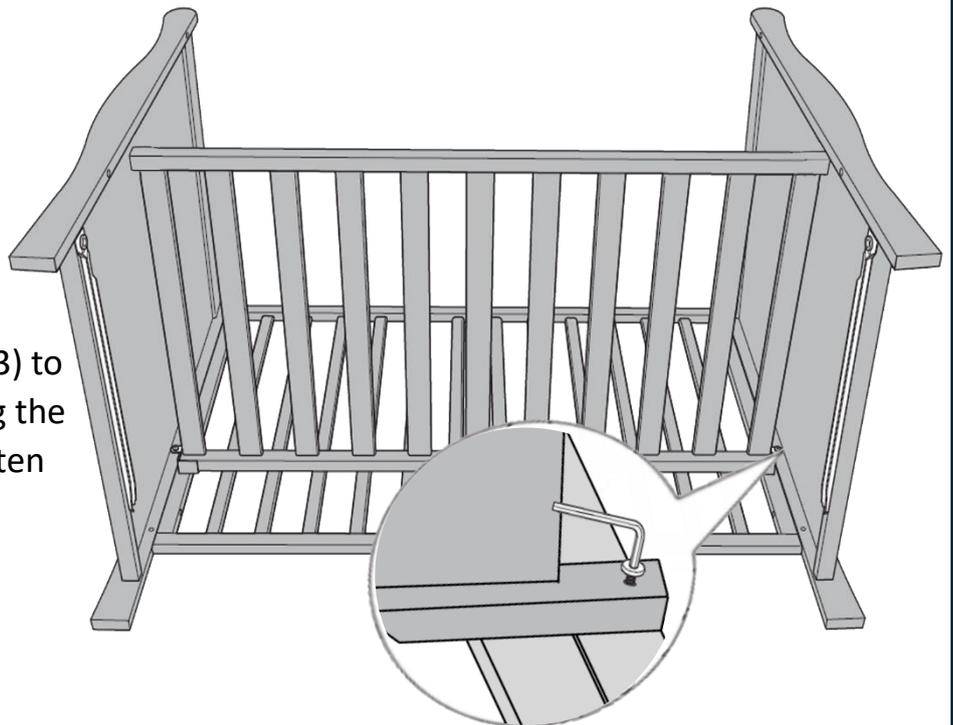
**NOTE: The Base Panel (3) can be adjusted as there are 3 height settings, the above shows the lowest.**
