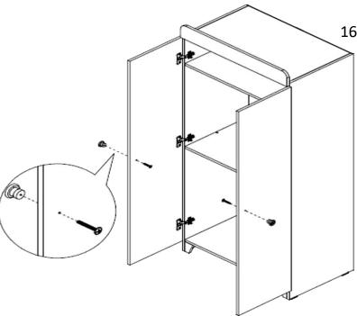
16. Attach the Door Handles (I) to the Wardrobe Doors (9), using the Handle Screws (A) and tighten with a cross-headed screwdriver not supplied.
