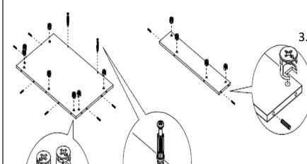
3. Attach Cam Lock Screws (D) into both the Top Panel (5). Insert both Cam Locks (B) and Wooden Dowels (C) into the corresponding slots on both the Top Panel (5) and the Top Back Panel (6).
