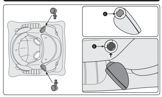
1. Insert the wing mirrors as shown, ensuring you line up the notched key on the underside of the mirror foot (A) with the notched keyhole on the walker body (B).
