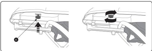
3. Secure the toy tray to the walker body by pushing the tabs (A) on the underside of the walker body, into the corresponding holes in the toy tray and then turning the tabs to fix the tray in position. Reverse the above process to remove the toy tray.
