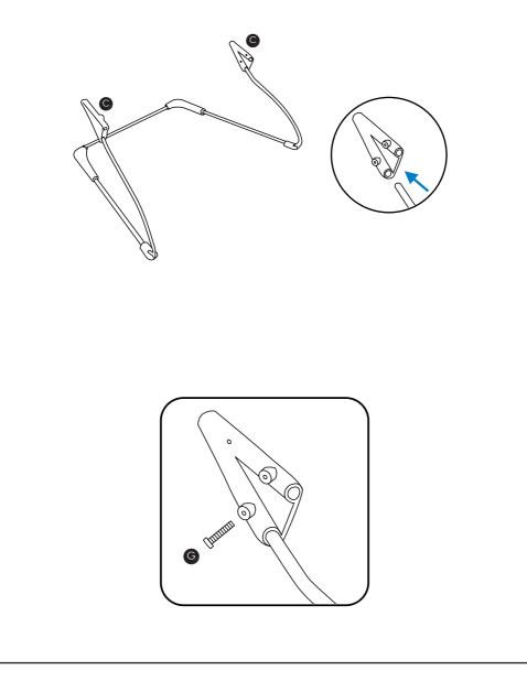
**6.4.** Fit both ends of the seat back frame (A) into the allocated holes in the seat back connector (B). Once connected fit both ends of the seat back frame (A) into the plastic connectors (C). Push the frame until the pin locks into the allocated holes.
