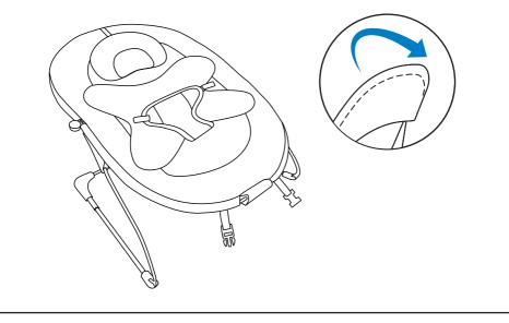
**6.8.** Slide the top of the vibration box (D) through the hole in the seat pad and onto the footrest frame. Fasten the clips under the seat.
