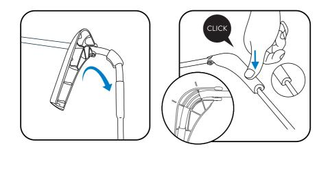
**6.3.** Fit left plastic connector (C) to the left support frame with the holes facing inwards and secure with screw (G). Repeat process to fit the right plastic connector (C) to the right support frame.
