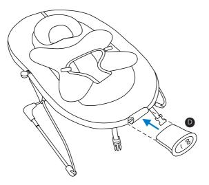
Fasten the clips under the seat. Reverse this process to remove the vibration box. NOTE. Ensure the vibration box has been fixed the right way up.
