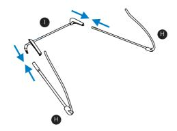
**6.2.** Lift the flip clip on both sides of the rear connector tube and lift the left support frame and right support frame into the rear frame tube. Close the flip clip over the tube and press down until the flip clips lock in place.
