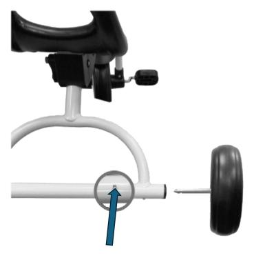
5. Attach the Rear Wheels (E) to the Chassis (A), slotting the wheel axle into the corresponding slot on the frame. Ensure that the Rear Wheels (E) click securely into place, gently pull the wheel to check.
