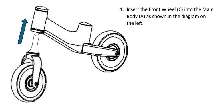
2. Place the Handlebar (B) down onto the Main Body (A) and it should click into place on the shaft of the Front Wheel (C). Pull up on the Handlebar (B) to check securely in place.
