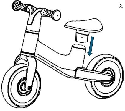
3. Insert the Seat (D) into the Main Body (A) as shown in the diagram on the left until it clicks into place. Pull up on the Seat (D) to check securely in place.
