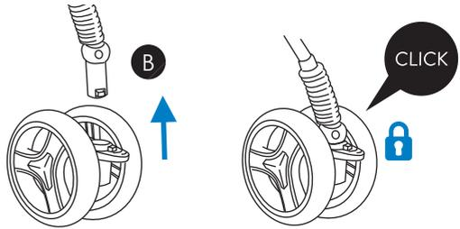
**To remove** locate the spring positioned between the wheels and squeeze to release.
