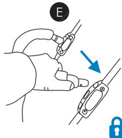
**To remove** the bumper bar, simply press the release buttons on both sides and lift off.
