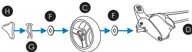
Attach the rear wheel axle (D) to the rear of the chassis. Push in until you hear a "click".
