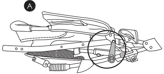
**HINT.** You may have to squeeze the stroller legs and handles together first so as to release the tension on the rivet.
